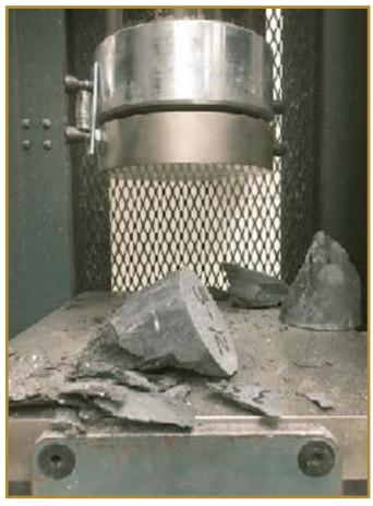
The final product must also hold up to Montana's harsh elements. During durability tests, the mixes were evaluated for alkali-silica reactivity, absorption, abrasion, chloride permeability, freeze-thaw resistance, and scaling. The mechanical and durability tests performed on the selected UHPC mix demonstrated exceptional mechanical properties and durability of this material.
