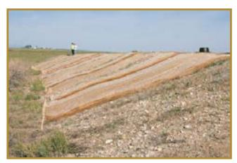
The ECBs included 2 weights of carded wool blankets, 2 types of needle punched wool blankets, and 2 different rolled ECBs of varying wool-straw ratios. The ECBs have variables such as density, thickness, strength, and amount of wool. Some resulted in greater desirable plant establishment than others. In general, the control plots had lower seeded grass canopy cover than all wool treatments except for the four-pass needle punch ECB.
