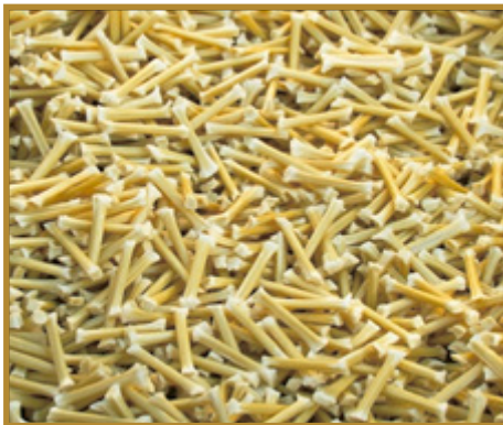
Sasobit Coated Aramid fibers
