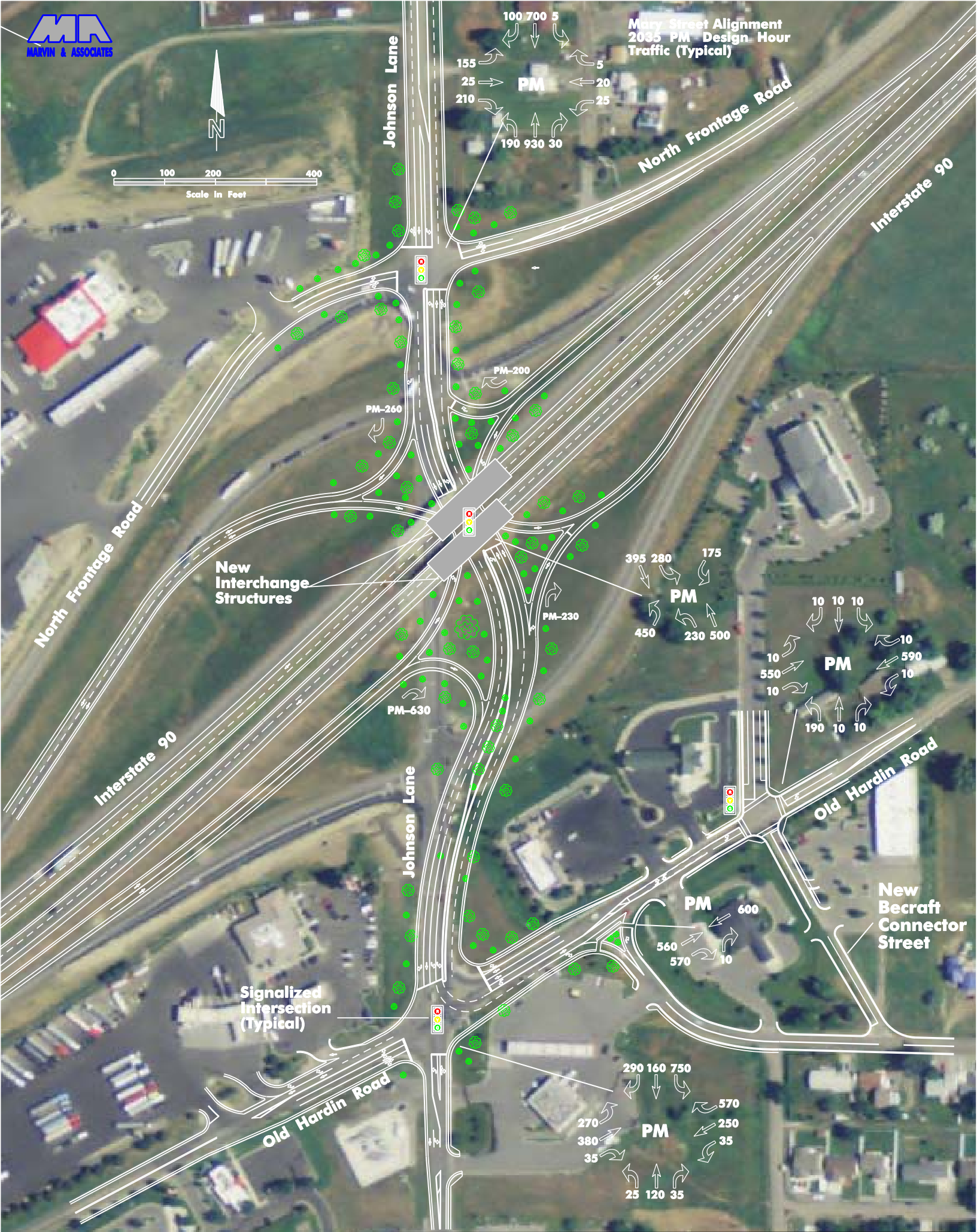
Figure H2. Single-Point Urban Interchange
