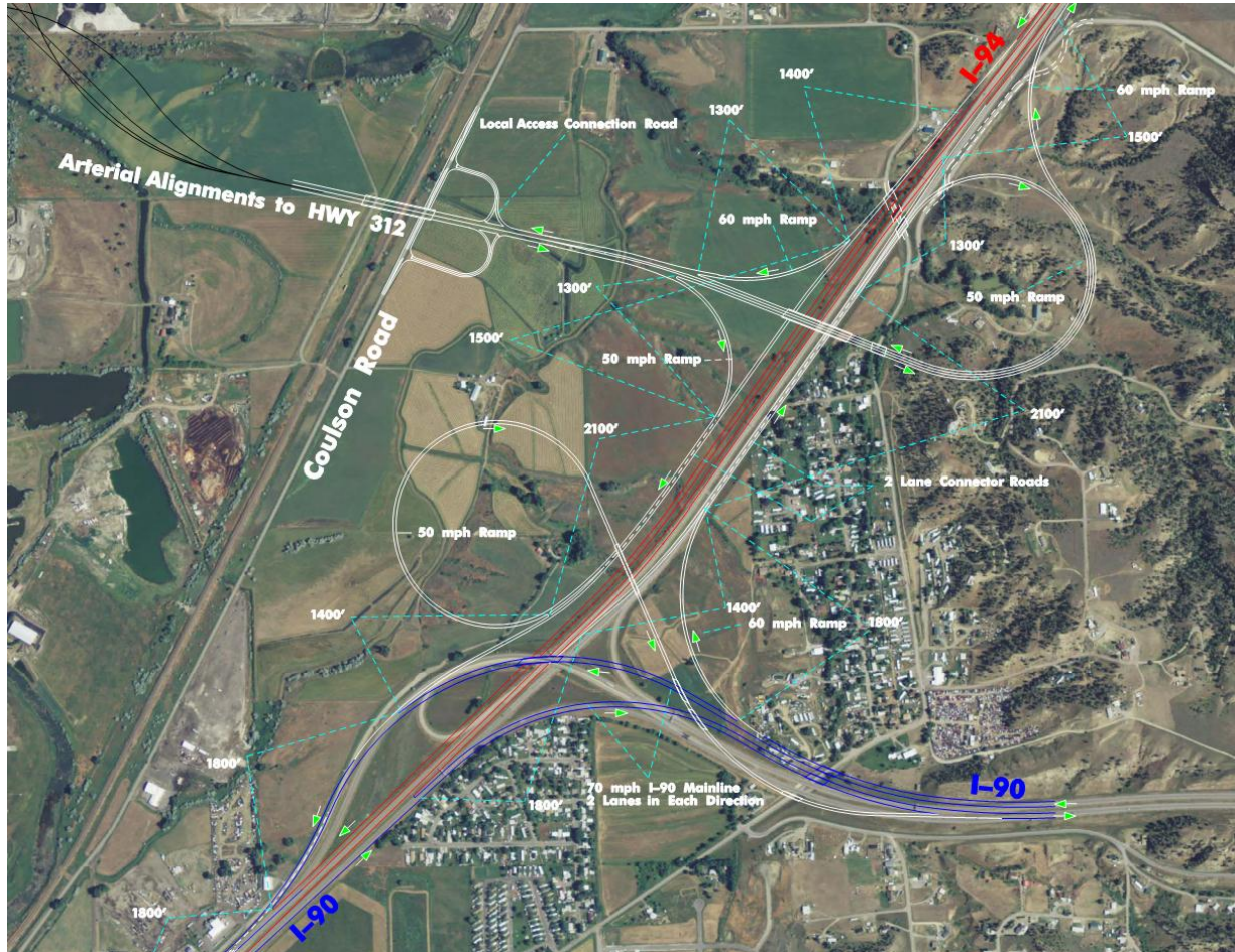
Figure 3.11 Pinehills Option 2 – Split Interchange
