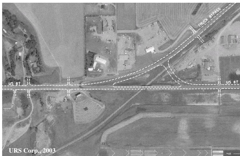
Figure 2-1 Bypass Junction – Alternative 2
