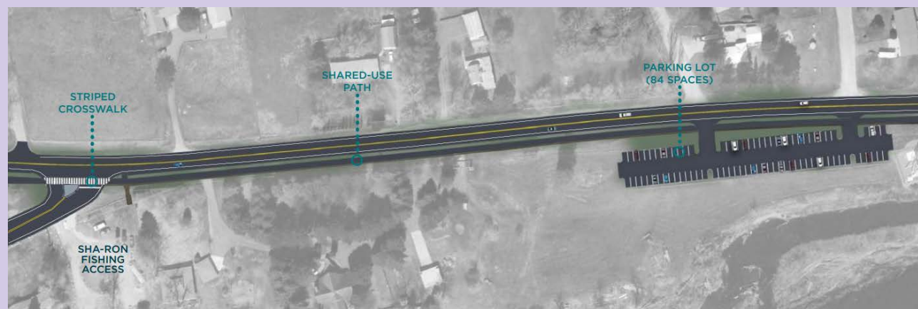
Preferred Highway 200 alternative includes a new parking lot within MDT right-of-way and a shared-use path connection to Sha-Ron fishing access
