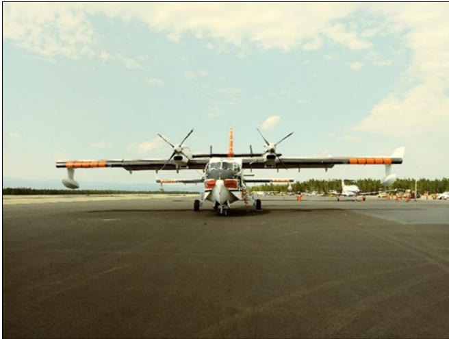
This CL-415 on the ramp at Yellowstone Airport can carry 1,600 gallons of water. See view of the water tanks from the interior of the plane in picture below.
