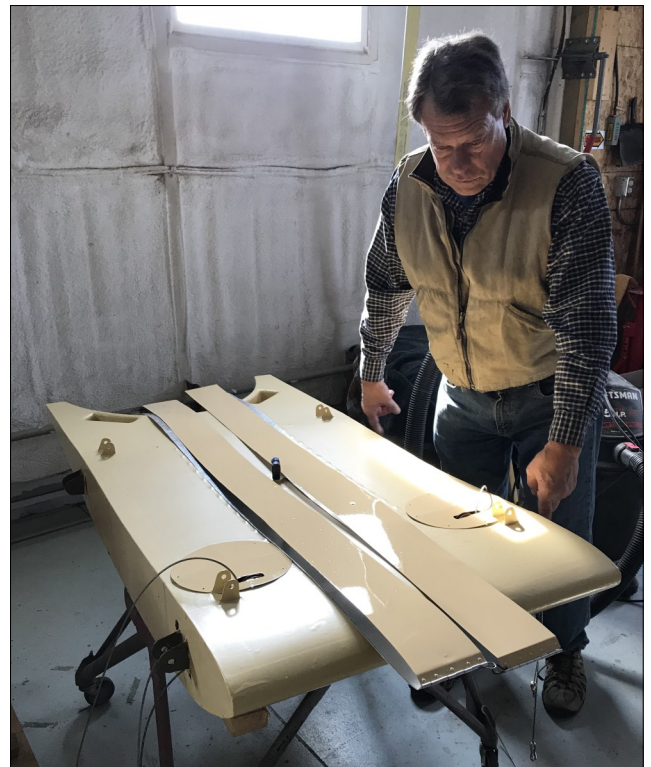
Paul Gordon explains how this wing center section will be installed on his Pietenpol Air Camper.
