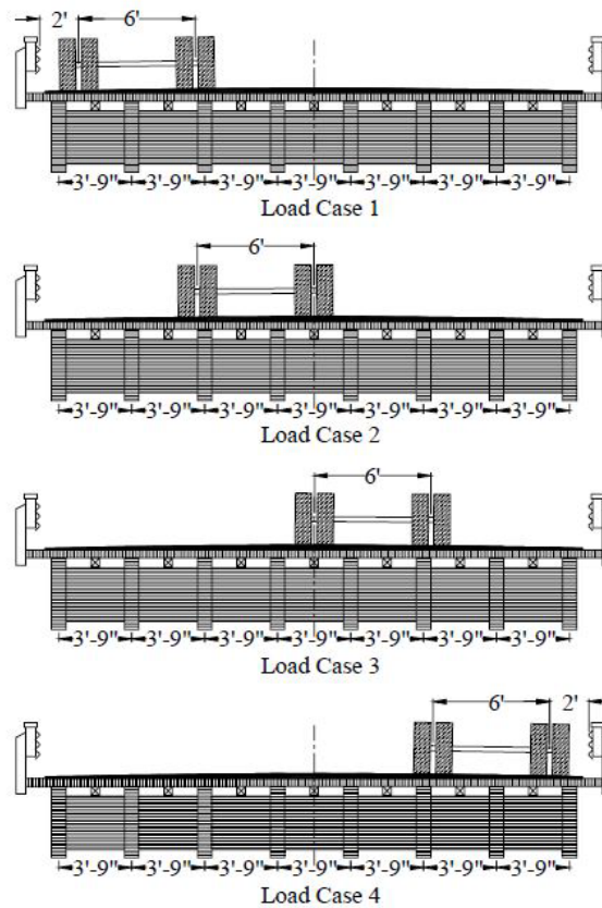
Figure 18: Load cases for Delaware county bridge [36].
