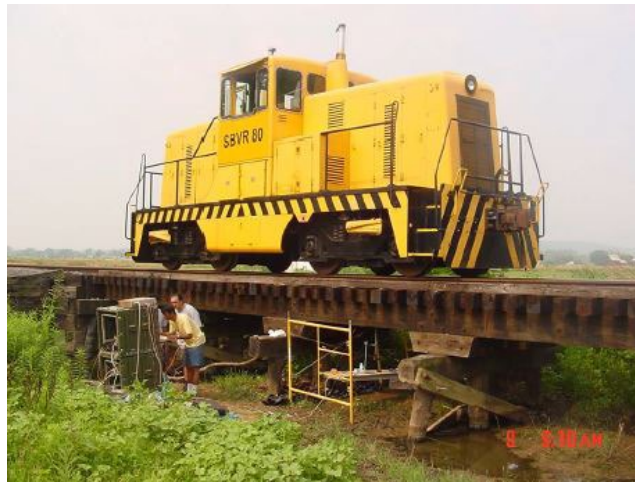
Figure 15: 80-TON SBVR Locomotive used for the Moorefield bridge field testing, West Virginia [35].
