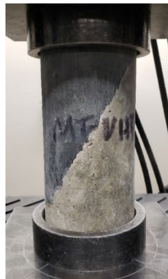
Figure 30: Slant-shear specimen in load frame
