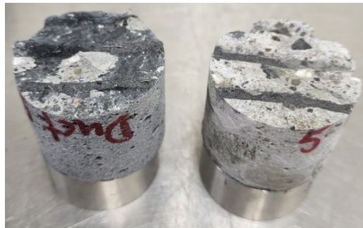
Figure 31: Example direct tension failure at the bond (Ductal-T Wet T1)
