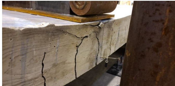
b) Concrete crushing prior to failing
