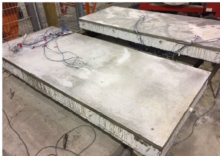
Figure 10: Example NC slabs with UHPC overlay and instrumentation [26]
