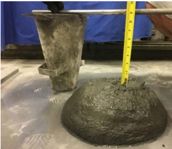
a) Slump Measurement
