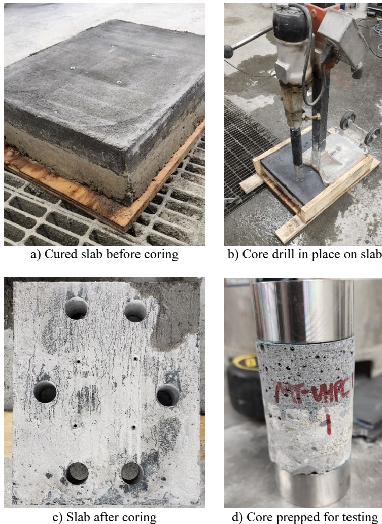
Figure 26: Typical direct tension core specimen preparation
