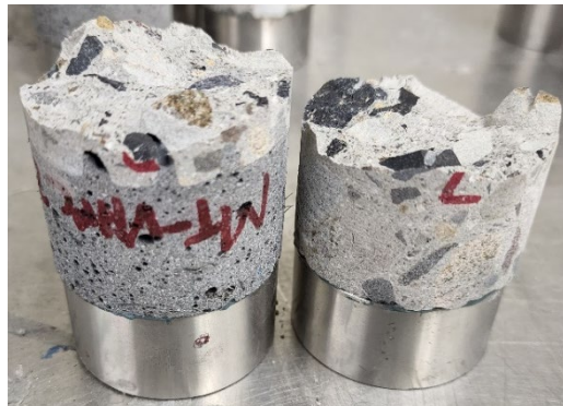
Figure 32: Example direct tension failure in the substrate concrete (MT-UHPC T2)
