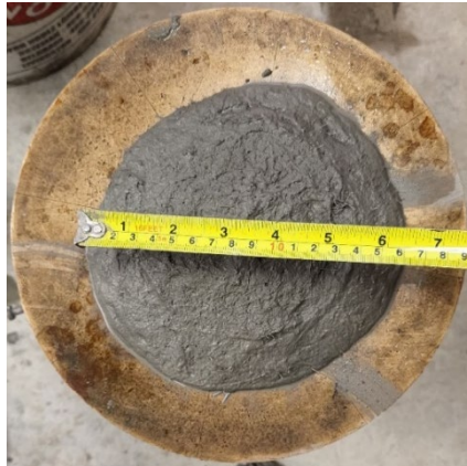
Figure 20: Dynamic flow test results for Ductal-T
