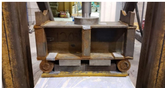
a) Load truck and steel plate
