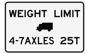
The new posting on the Twelve Mile Creek Bridge applies to SHVs; it limits the maximum gross vehicle weight of single-unit vehicles with 4, 5, 6, or 7 axles to 25 tons.
