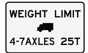
The new posting on the US 12 Drainage Bridge applies to SHVs; it limits the maximum gross vehicle weight of single-unit vehicles with 4, 5, 6, or 7 axles to 25 tons.
