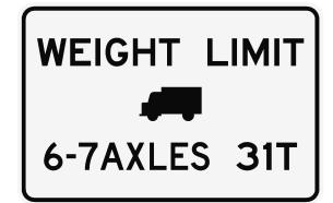
The new posting on the South Fork People's Creek Bridge applies to SHVs; it limits the maximum gross vehicle weight of single-unit vehicles with 6 or 7 axles to 31 tons.
