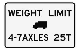
The new posting on the Coffee Creek Bridge applies to SHVs; it limits the maximum gross vehicle weight of single-unit vehicles with 4, 5, 6, or 7 axles to 25 tons.
