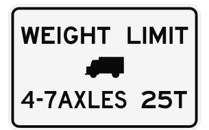
The new posting on the Pondera Coulee Bridge applies to SHVs; it limits the maximum gross vehicle weight of single-unit vehicles with 4, 5, 6 or 7 axles to 25 tons.
