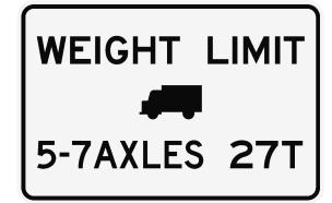
The new posting on the MacDonald Creek Bridge applies to SHVs; it limits the maximum gross vehicle weight of single-unit vehicles with 5, 6, or 7 axles to 27 tons.
