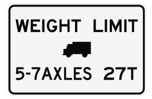
The new posting on the Smoke Creek Bridge applies to SHVs; it limits the maximum gross vehicle weight of single-unit vehicles with 5, 6, or 7 axles to 27 tons.
