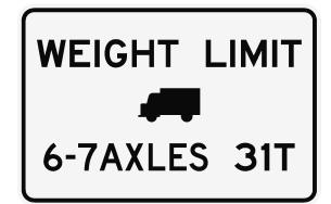
The new posting on the Redwater River Bridge applies to SHVs; it limits the maximum gross vehicle weight of single-unit vehicles with 6 or 7 axles to 31 tons.
