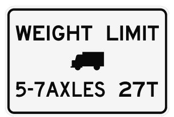
Bridge weight restrictions are required when the engineering analysis of a bridge, known as a load rating, indicates that it cannot carry standard, legal loads. Load ratings provide information about how much distributed weight can safely pass over a bridge. Load posting signs show maximum weight limits for different vehicle types, depending on their axle configuration. A posted bridge is safe to use, but the weight of certain vehicles must be limited accordingly.
