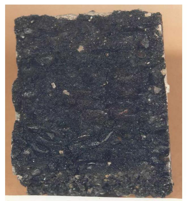
MOISTURE DAMAGED (3) LOSS OF SHEEN, DULL APPEARANCE SOME SMALLER AGGREGATE (-10 M) IS UNCOATED
