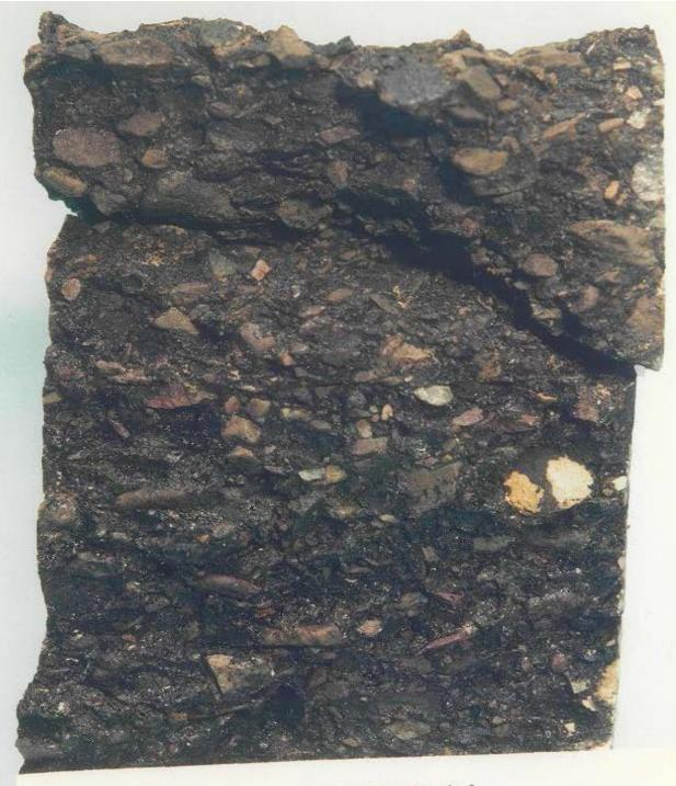
SEVERLY STRIPPED (1) MOST OF THE AGGREGATE IS SO CLEAN THE COLORS OF THE ROCKS ARE EASILY SEEN
