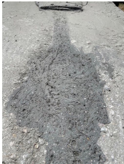
Figure 38: UHPC surfaces ground after a 6-hr cure time
