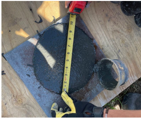
Figure 32: Flow test of MT-UHPC during mockup
