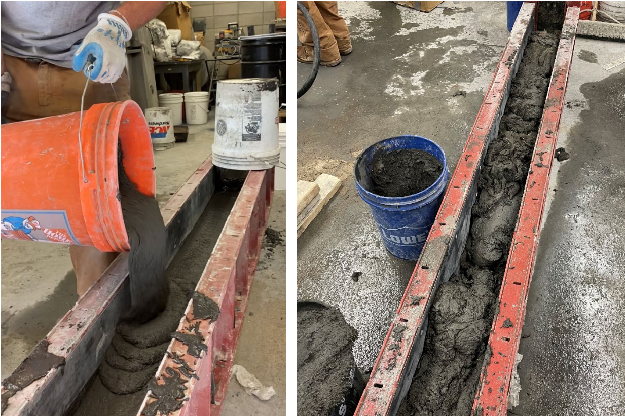
(a) successful 4.5 ft 3 batch being placed
