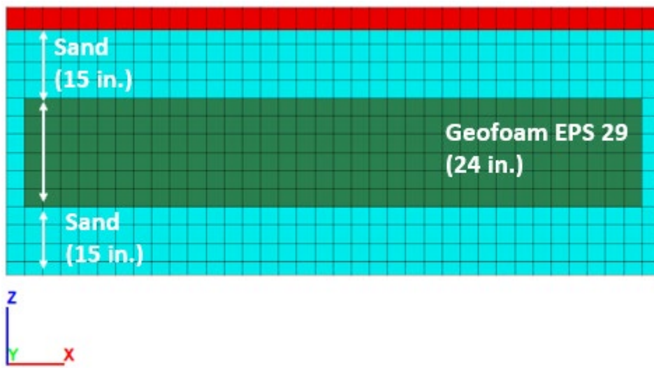
Figure C39. A cross-section in X direction for scenario 20-Geofoam EPS 29 (24 in. thick in Z direction).
