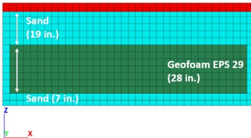
Figure C47. A cross-section in X direction for scenario 24-Geofoam EPS 29 (28 in. thick in Z direction).
