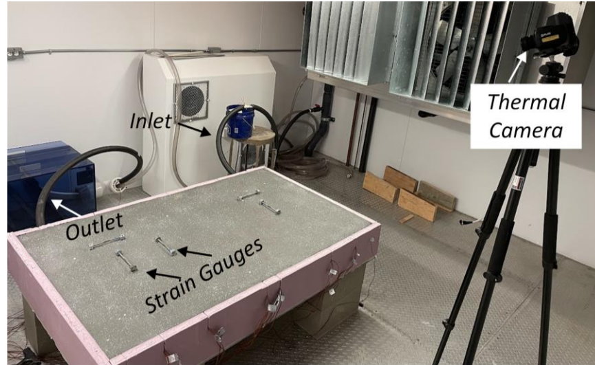
Figure 16. Bridge deck model prepared for testing
