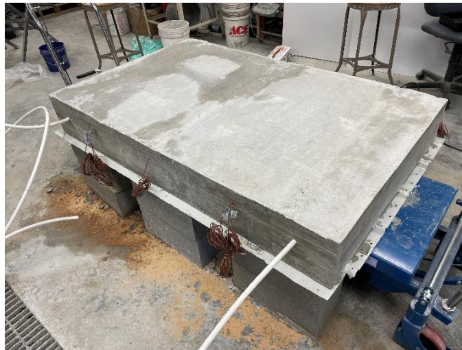
Figure 14. Cured bridge deck model
