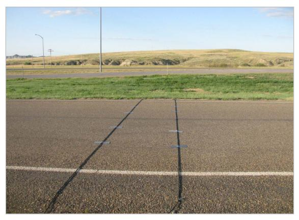
Figure 3-3: Pneumatic Tube Setup
