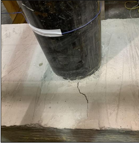
Figure 47: VT2/3-4U first cracks (92 k-ft)
