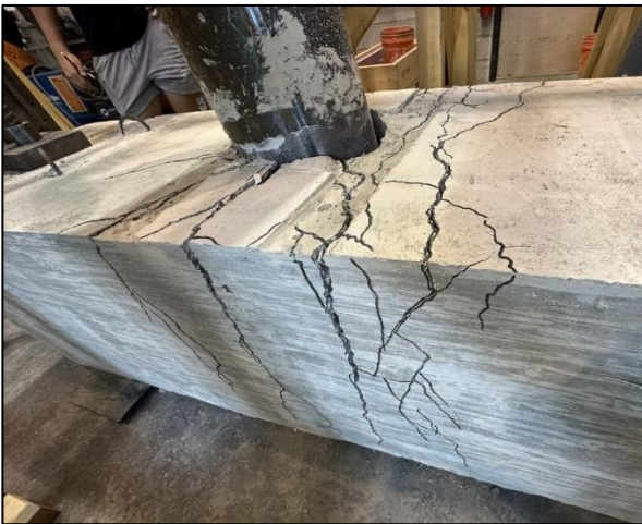
Figure 43: VT2/3-6 failure from initial loading direction
