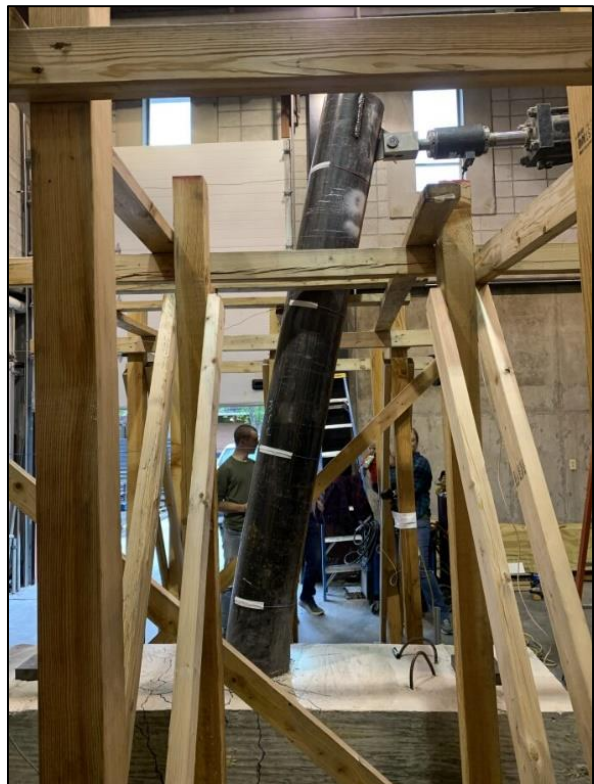
Figure 50: VT2/3-4U failure from initial pull direction
