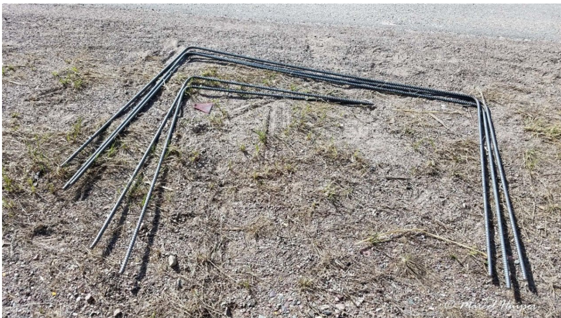
Figure 6: Several of the “staples” (60-inch horizontal, 107 cm (42 inch) legs) the L-shaped corner elements (91 cm (36 inch) swing arms, 107 cm (42 inch) legs).
