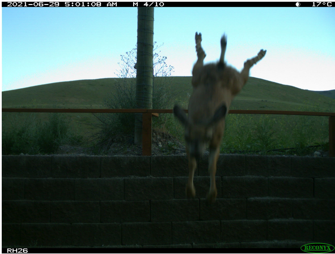
Figure 12: A mule deer jumps down the jump-out with the prototype (height 46 cm (18 inches), setback 10 cm (4 inches)). The animal starts the jump from behind the bar and does not step over the bar first before jumping down.
