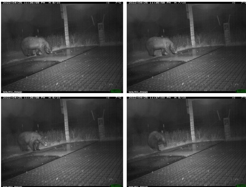
Figure 14: A black bear approached the wildlife guard and electrified barrier (BS Fabrications). Based on the images, this animal was shocked and ran back to the habitat side.
