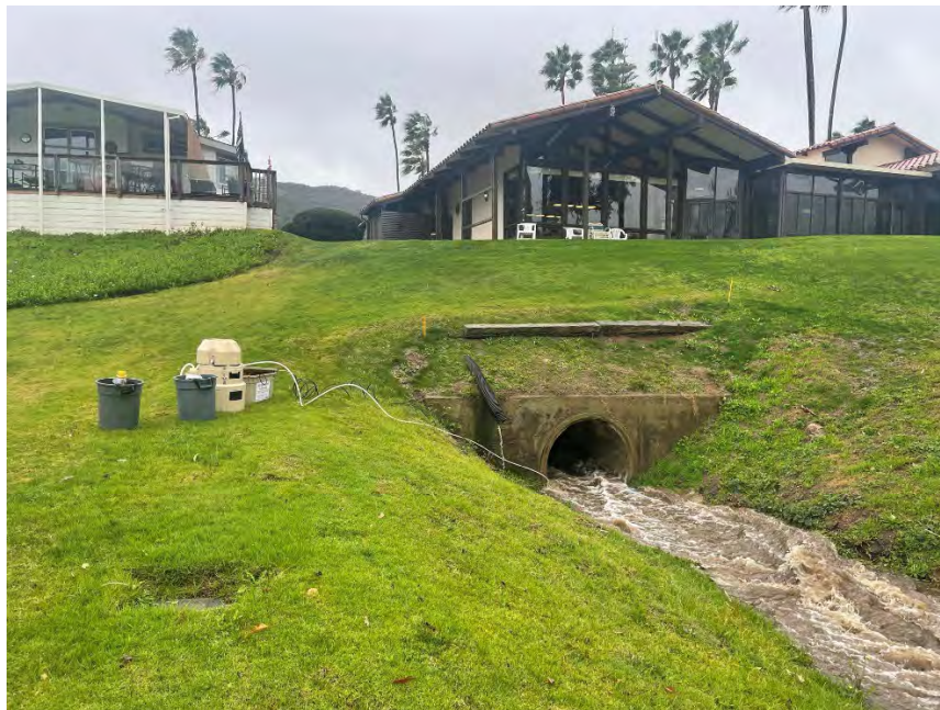
Figure 4-8a. Example of Temporary Automated Sampler Setup
