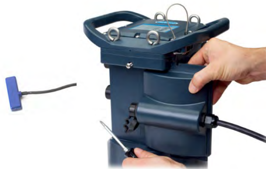
Figure 4-4. Hach® Submerged AV Sensor and FL900 Logger with AV9000 Analyzer Module
