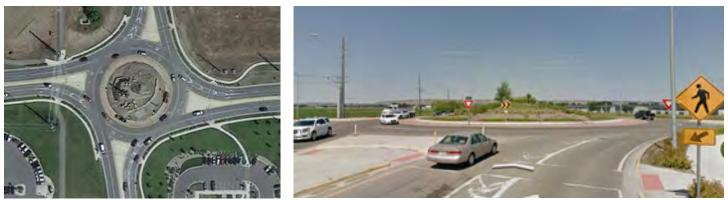
Figure 10.13: Hybrid Multi-lane Roundabout (2x1) – E North Pacific Avenue and Airway Boulevard, Belgrade, MT
