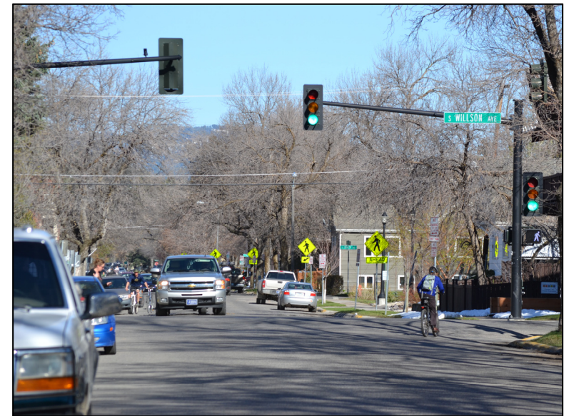
Bicycle level of traffic stress (LTS) is determined based on factors including posted speed limit, street width, and the presence and character of bicycles lanes.
