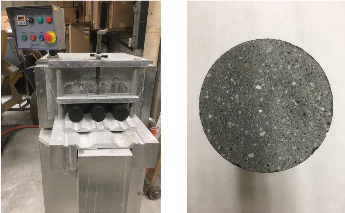
**Figure 4: Cylinder end grinder and prepared test specimen**
