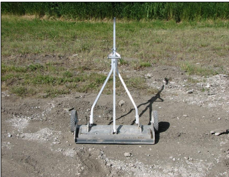
← A magnetic sweeper is used to remove any remaining metal shot on the deck surface.
