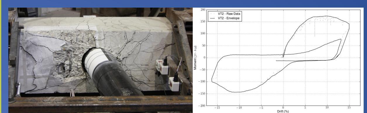
VT2 - oversized pile with significant cap deterioration
