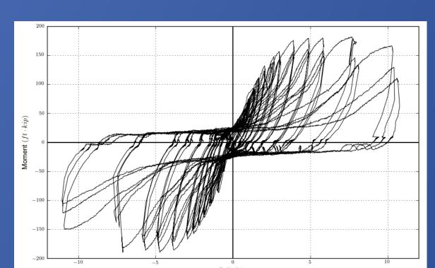
CT2 - oversized pile with significant cap deterioration
