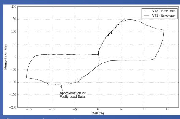
VT3 - oversized pile with significant cap deterioration
