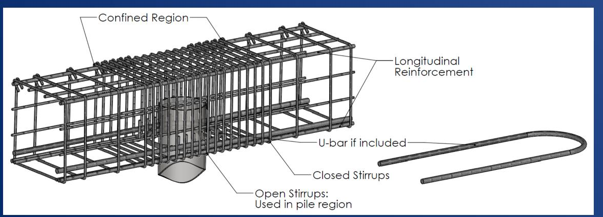
Example of improved connection reinforcement scheme with U-bars
