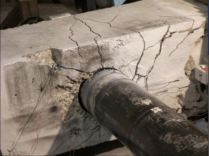
Example of test specimen VT2.5 with degraded concrete cap – Non-Ductile Behavior with pinched hysteresis response
