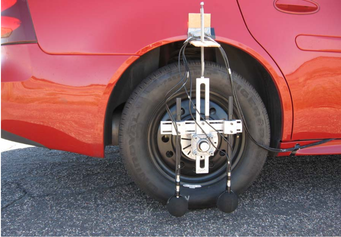
Figure 1. OBSI Equipment Installed on a Test Vehicle
