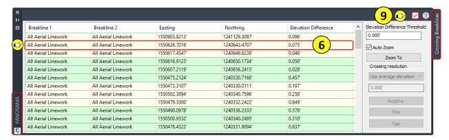
All identified crossing breaklines are listed in the **Crossing Breaklines** PANORAMA vista. The various available elevations options can be used to resolve the Crossing Breaklines.
