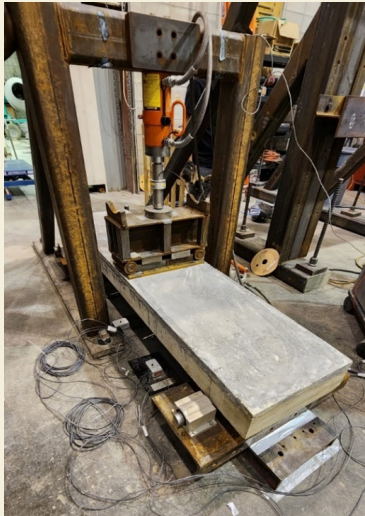
Figure 2: UHPC overlay slab test set-up.
