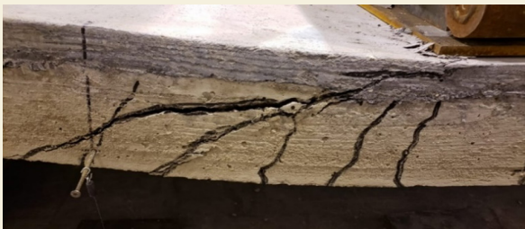
Figure 4: Shear failures of the positive moment UHPC overlay slab specimens.
