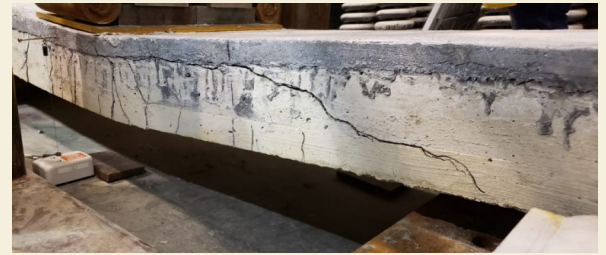
Figure 4: Shear failures of the positive moment UHPC overlay slab specimens.
