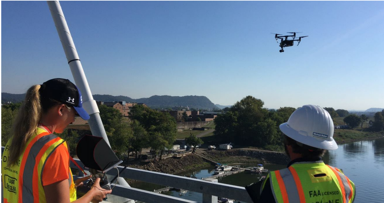
Figure 3.7.1-1 A UAS pilot and a sensor operator fly a UAS to collect video on a cable.
