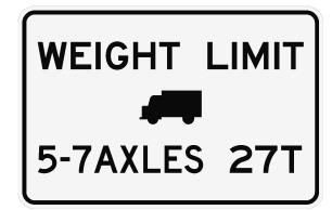
The new posting on the MT 200 Drainage Bridge applies to SHVs; it limits the maximum gross vehicle weight of single-unit vehicles with 5, 6, or 7 axles to 27 tons.
