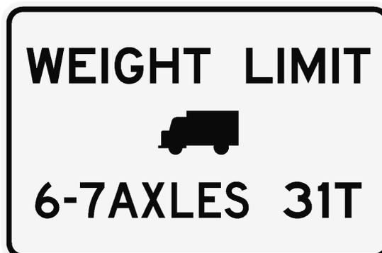
The new posting on the Redwater River Bridge applies to SHVs; it limits the maximum gross vehicle weight of single-unit vehicles with 6 or 7 axles to 31 tons.
