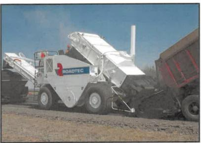
The SB-2500B Shuttle Buggy® material transfer vehicle can store and transfer hot-mixed asphalt material from a truck to a paver for continuous paving. A patented antisegregation auger remixes materials just before they are delivered to the asphalt paver. The 25-ton (22.7 MT) surge capacity of the SB-2500B allows trucks to unload material immediately and return to the asphalt plant. Options include the windrow pickup head and the road widener attachment.
