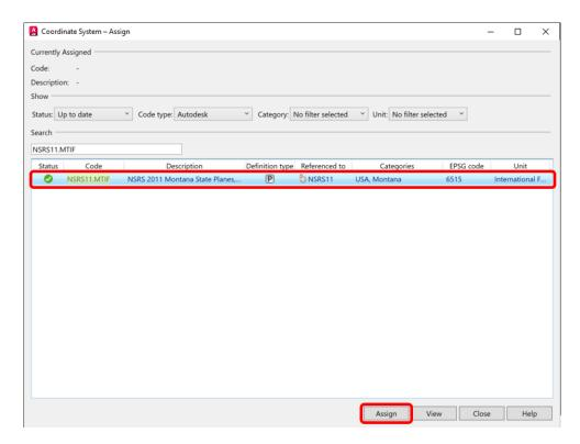
g. The coordinates icon located on the bottom ribbon will populate to display the assigned coordinate system.
