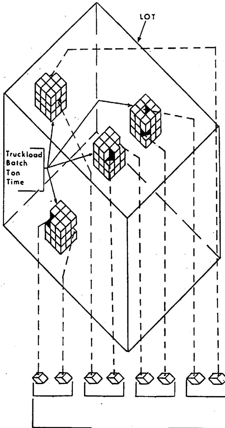
**FIGURE 1**—Schematic diagram illustrating *Lot, Sample, Subsample, and Sample Unit.*
