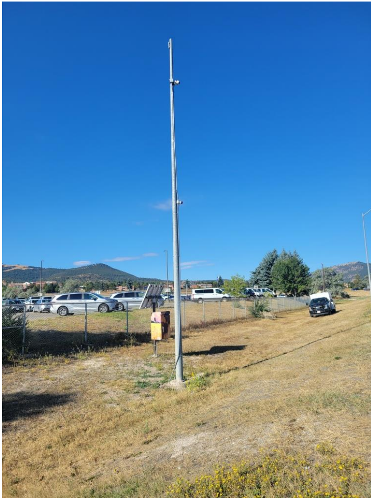
Figure 12 Leetron Video Counter (Non-Intrusive) at Prospect Ave (US 12), W of Gibbon St Source: Montana Department of Transportation, 2014
