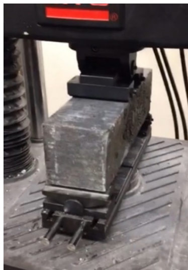
Figure 10: Flexural test specimen in load frame
