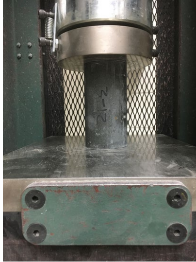
Figure 9: Compression cylinder in load frame
