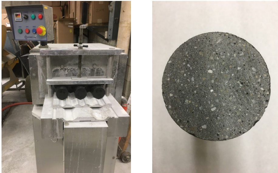
Figure 8: Cylinder end grinder and prepared specimen
