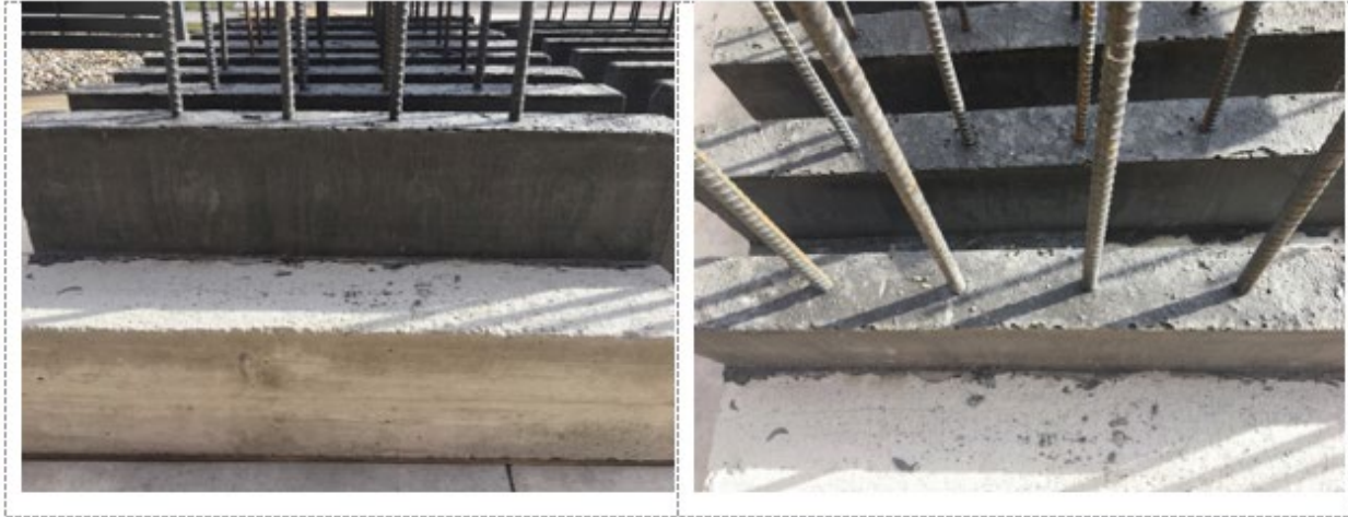
Figure 30: FHWA Recommended tests 14 through 16 showing no UHPC effect as test results ended with rebar yielding
