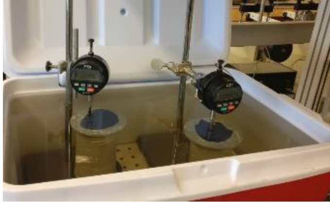
Figure 5.8: Moisture conditioning by submerging the specimen.
