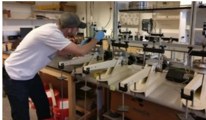
Figure 11.4: Sample setup for the 1-D swell test
