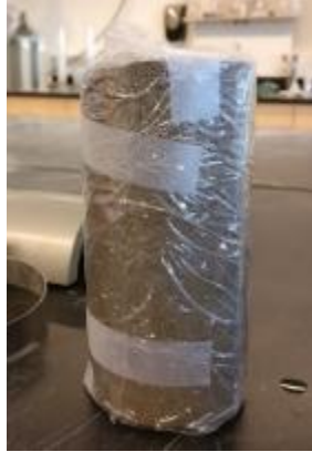
Figure 5.1: Sample wrapped in cellophane sheet to ensure no loss of moisture
