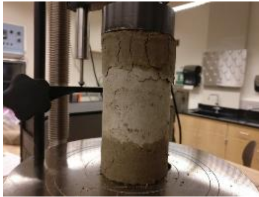
Figure 5.9: UCS testing of an accelerated cured sample.
