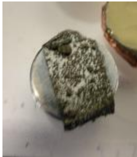
Figure 4.9: Carbon coated sample for SEM imaging
