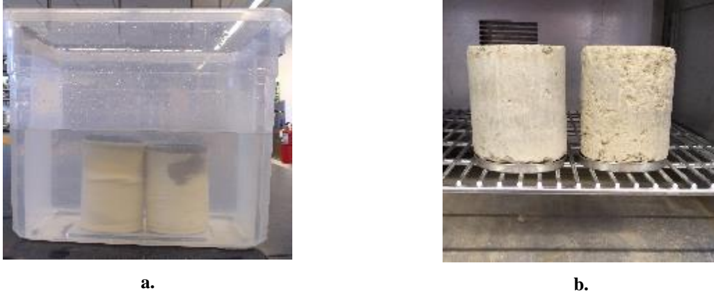
Figure 6.2: W/D Testing Cycles – a) Wetting Cycle b) Drying Cycle
