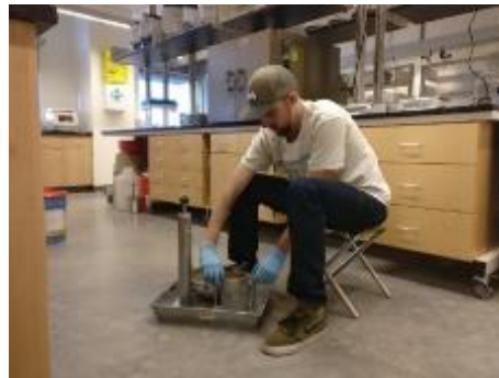
Figure 11.2: Proctor Test on BR soil
