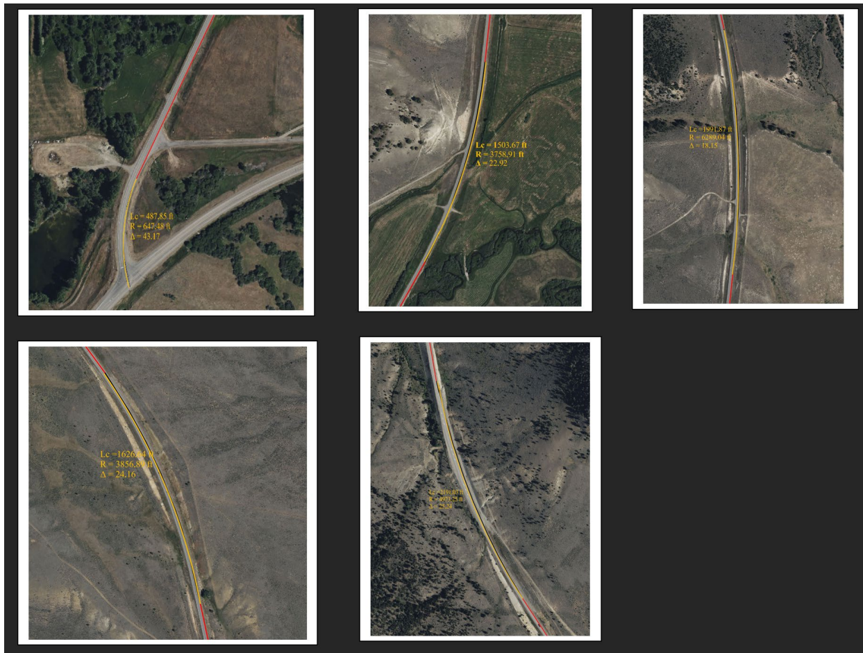
Figure 7. Verifying the radius and length of curves for route C00060A using Geolocation feature in Civil3D
