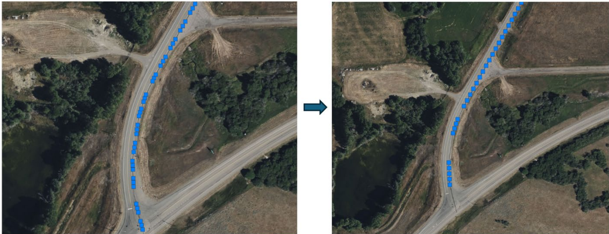
Figure 4. Segments before joining (left) and after joined together (right) based on the change in bearings
