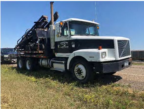
Heavy truck used for testing: 2000 Volvo Model 999 Truck Tractor, diesel powered, manual transmission, approx. GVW 18,000 lbs. plus drill equipment.
