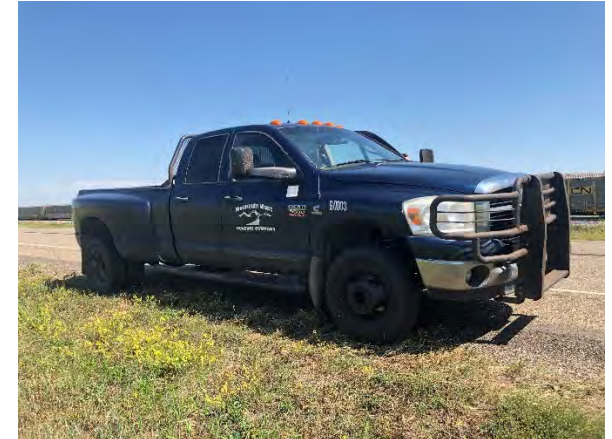
Medium truck used for testing: 2007 Dodge Ram Dually 3500 Quad Cab, diesel powered, manual transmission approx. GVW 11,000 lbs.
