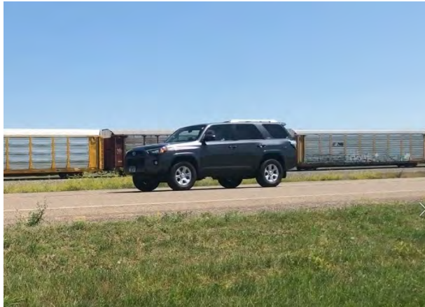
Passenger vehicle used for testing: 2018 Toyota 4Runner, gas powered, automatic transmission, approx. GVW 6,100 lbs.
