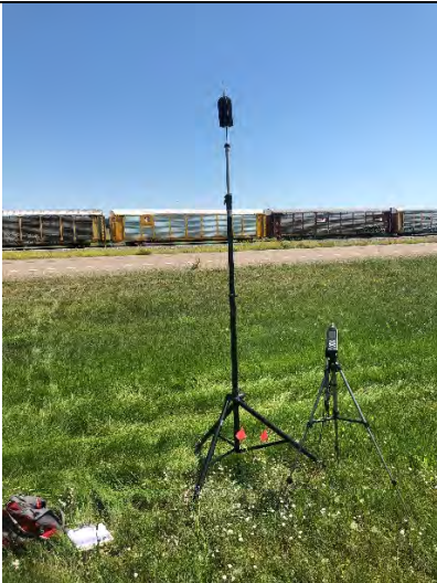
Looking east at representative SLM and microphone equipment set up in MT-39 ROW 50 feet from centerline (measurement location SCLRS S3A).
