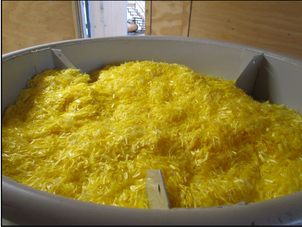
↑ View of the aramid fibers loaded in the hopper.
