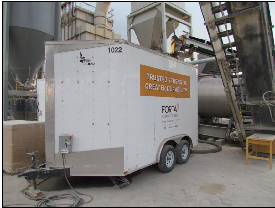
↑ The required automated feeding system was contained in an enclosed trailer that was parked near the hot plant.
