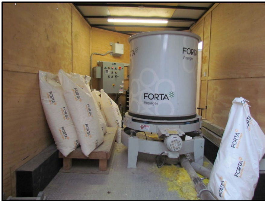
↑ This trailer included a hopper and feed line as well as controls for the feed system. The hopper had a 300 lb capacity. The technician would input the desired weight of fibers and the production rate of the hot plant and using that information the control board would spin the hopper which would deposit fibers into the feed tube that would then deposit the fibers into the hot plant drum to mix with the plant mix.
