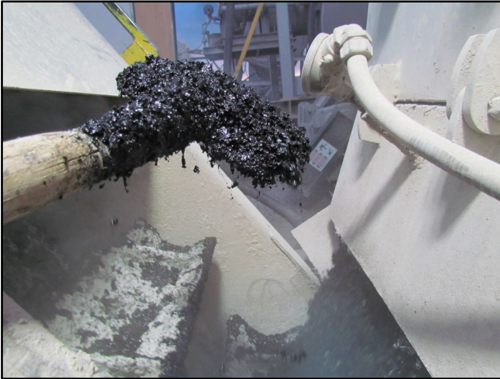
↑ Example of the plant mix surfacing deposited out of the hot plant. Notice the fibers hanging from the mix.
