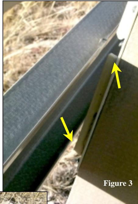
As noted in the October 2000 Report. The right, rear bolt attachment to the frame sill has broken (Figure 4). During this investigation, it was observed the sill had jumped once more to the left of the broken bolt of the rear ground support. This
