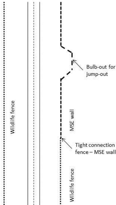
**Figure 6: Fenced road corridor with jump-outs integrated into MSE wall through a bulb-out.**
